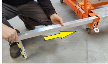
Figure 11. Inserting the rotated stabiliser feet
