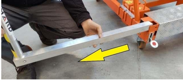
Figure 10. Pulling out the feet from the socket
