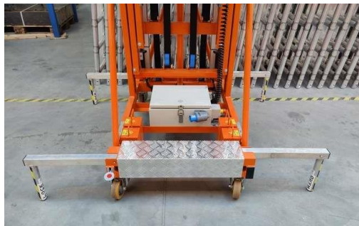
Figure 14. Unfolded the side stabiliser feet
